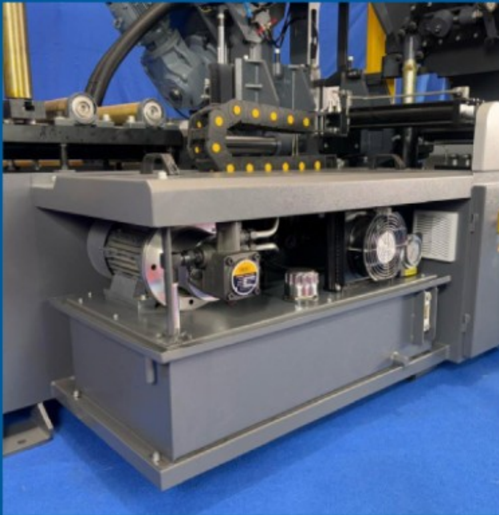
Hydraulic power pack air coolers are designed to maintain optimal oil temperature for efficient system performance. They enhance the durability and reliability of hydraulic components by preventing overheating. Compact and robust, they are ideal for continuous industrial operations
