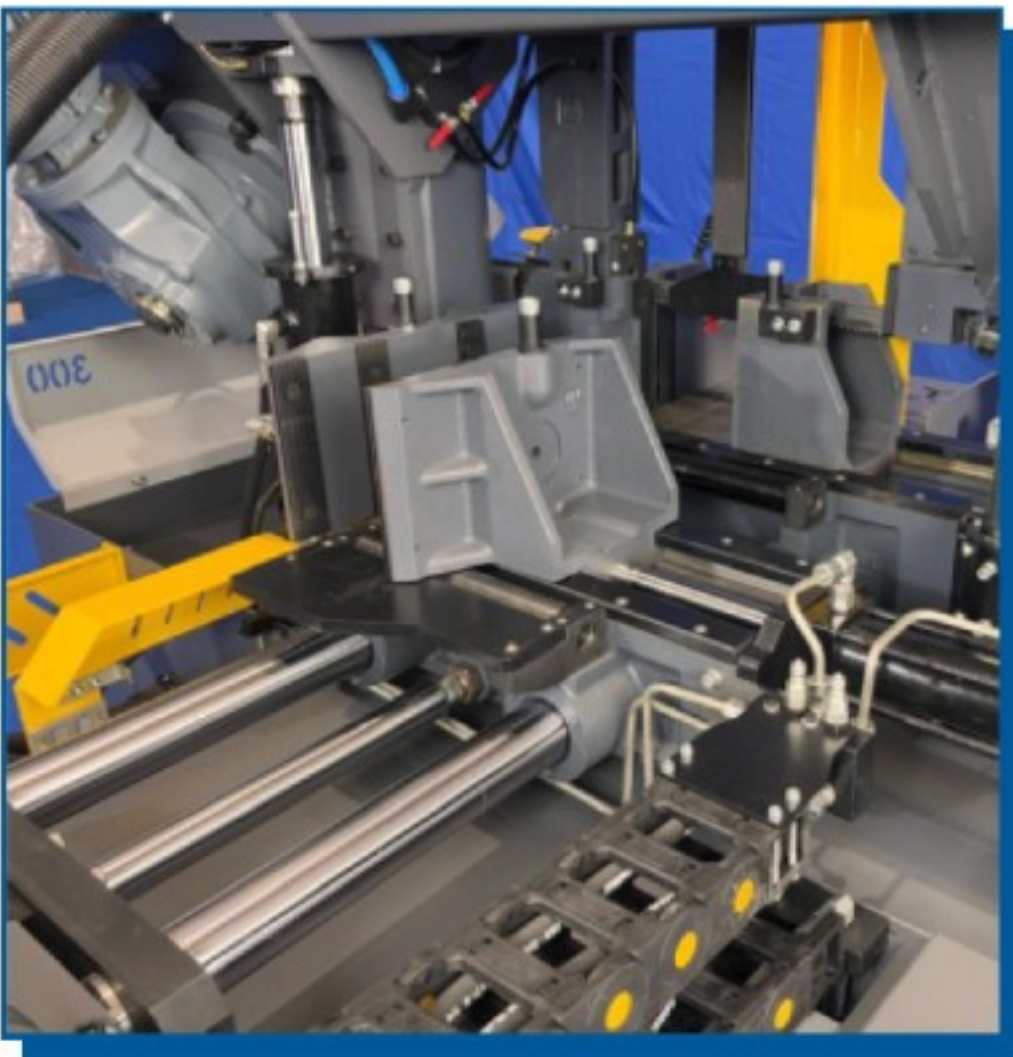
"Equipped with an automatic bandsaw indexing table featuring a floating vice for superior length accuracy. Ensures precise material positioning with minimal clamping force variations. Enhances cutting efficiency and consistency for long work pieces."
