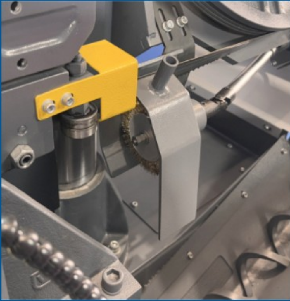
Power drive chip brushes are essential for removing chips and debris from the cutting area, ensuring smooth operation. Designed for durability and efficiency, they maintain the blade's performance and longevity. Ideal for keeping bandsaw machines clean and precise.
