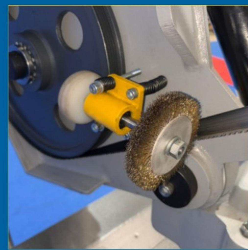
Power drive chop brushes are essential for removing chips and debris from the cutting area, ensuring smooth operation. Designed for durability and efficiency, they maintain the blade's performance and longevity. Ideal for keeping bandsaw machines clean and precise.
