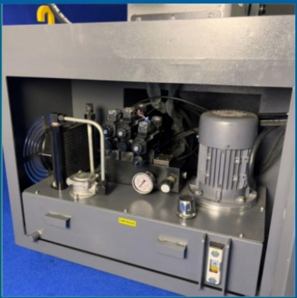
Hydraulic power pack air coolers are designed to maintain optimal oil temperature for efficient system performance. They enhance the durability and reliability of hydraulic components by preventing overheating. Compact and robust, they are ideal for continuous industrial operations.
