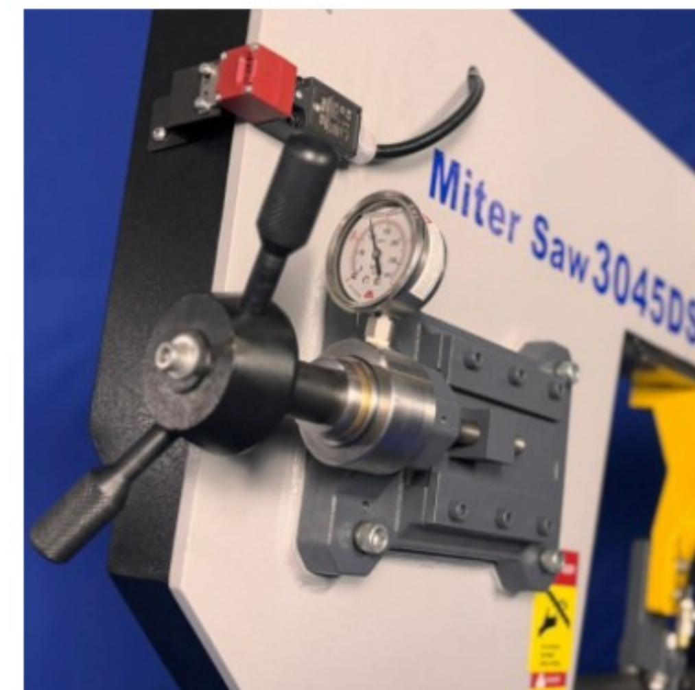
Features a manual blade tensioning system with a hydraulic pressure gauge for precise adjustments. This ensures accurate blade tension for optimal cutting performance. Achieve consistent results with easy and reliable tension control.
