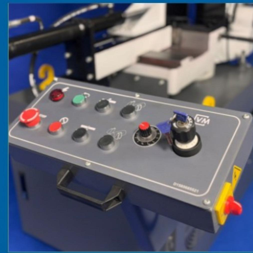
"Movable control panel with push-button dashboard for easy and flexible operation. Allows multi-angle access, ensuring user convenience and efficient machine control."
